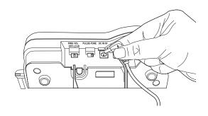
2. Place the AC Adapter cord inside the molded channel.
